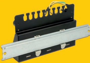
43339 ● 43335 ○ Keystone Desktop Patch Panel 12 Port • 12 Keystone ports 19.2 x 14.9 mm • Cable routing 180° • Colour: jet black RAL 9005 • Metal housing • Shielded • 2 DIN-rail clips
